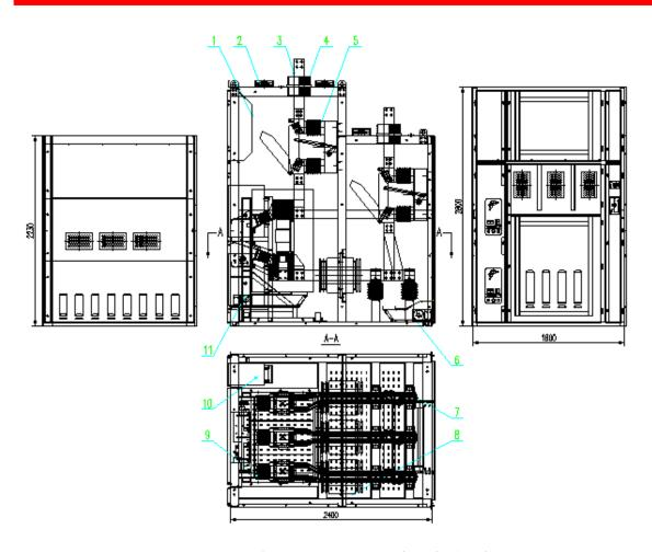
Structure of the Switchgear
