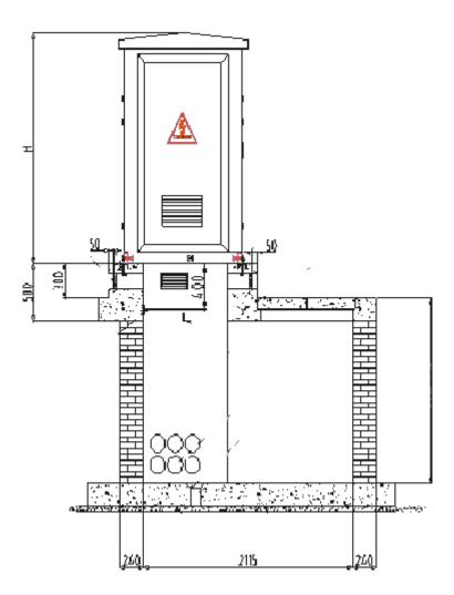
To ensure the installation quality of the foundation construction, the outdoor housing base installation requirements are 5mm/m., check whether all fastening bolts are loose or not, and whether the wiring is reliable.
